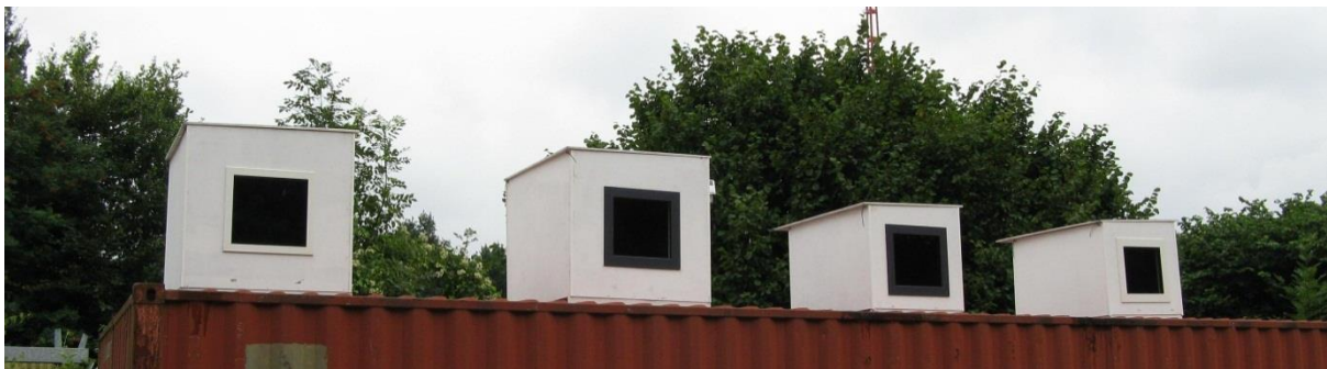
Figure 5-2: Four insulated boxes containing concrete floors, with and without PCMs, as part of the experimental set-up at the University of Twente.
